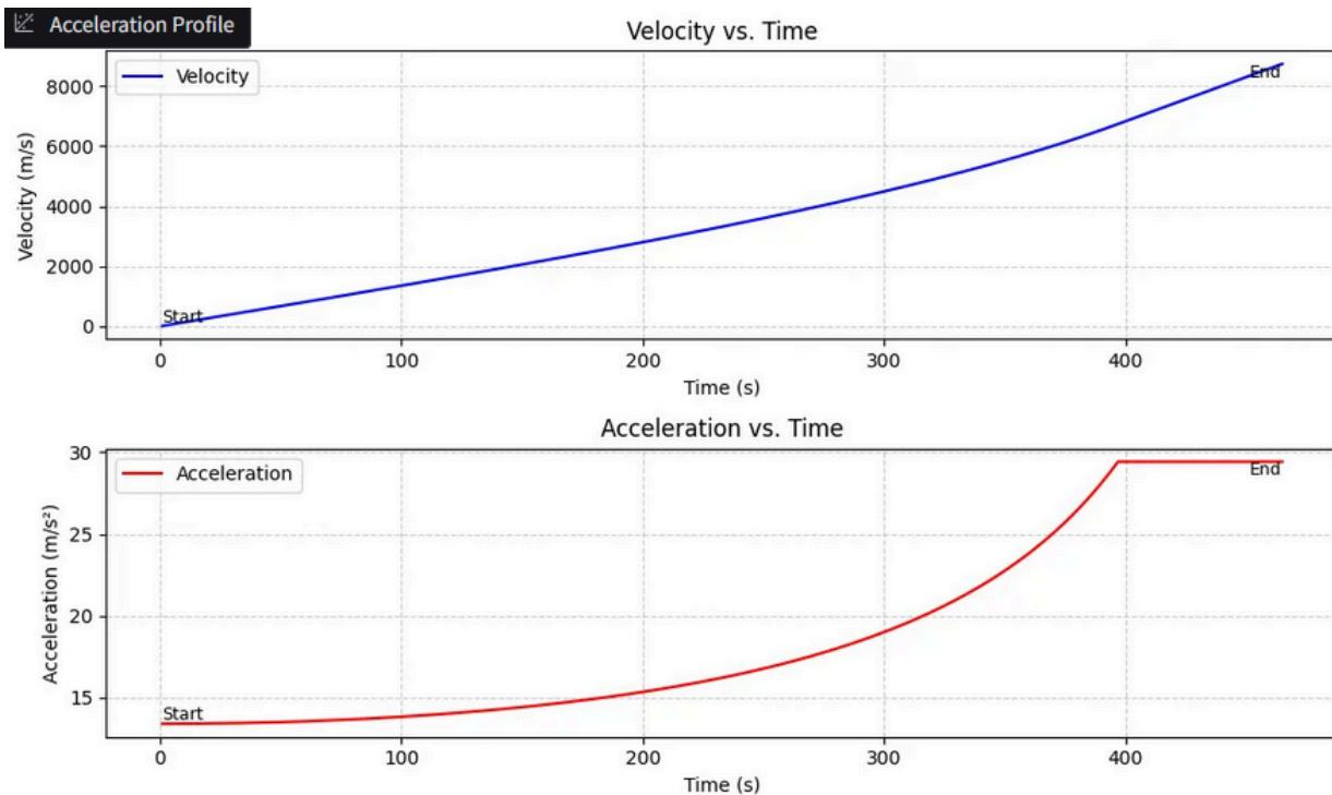
A tether with uniform width and thickness cannot pull by the full  $3g$ 's we desire until most of its mass is reeled in. The area of the tether is too small at the start and too large at the end. How can we improve this?
