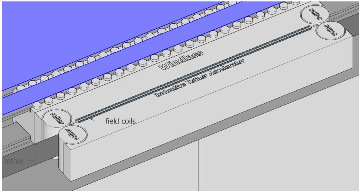
For a reel 12.57 kilometers in circumference, a 1700 km tether would wrap 135ish times and be about 2 meters thick.
