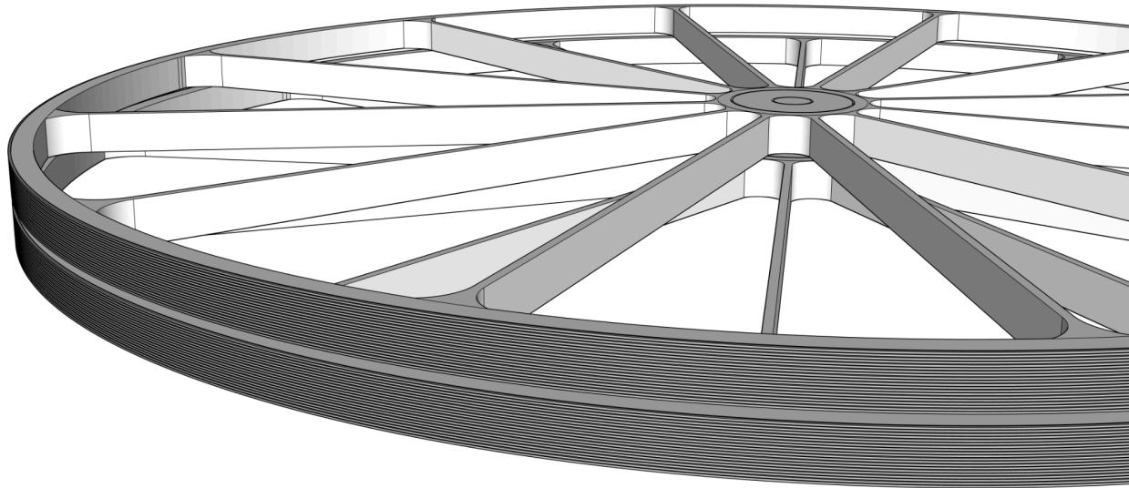
With the high width to height ratio of the flywheels, up to half a dozen flywheels can share an axel before stability is an issue. Stacking flywheels on a common axis allows them to exchange power and inertia and share stationkeeping infrastructure.
