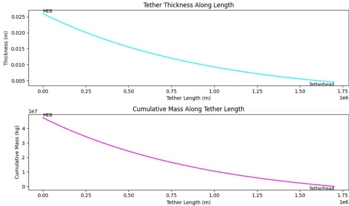
The area under the curve is the total mass of the tether we calculated previously.
