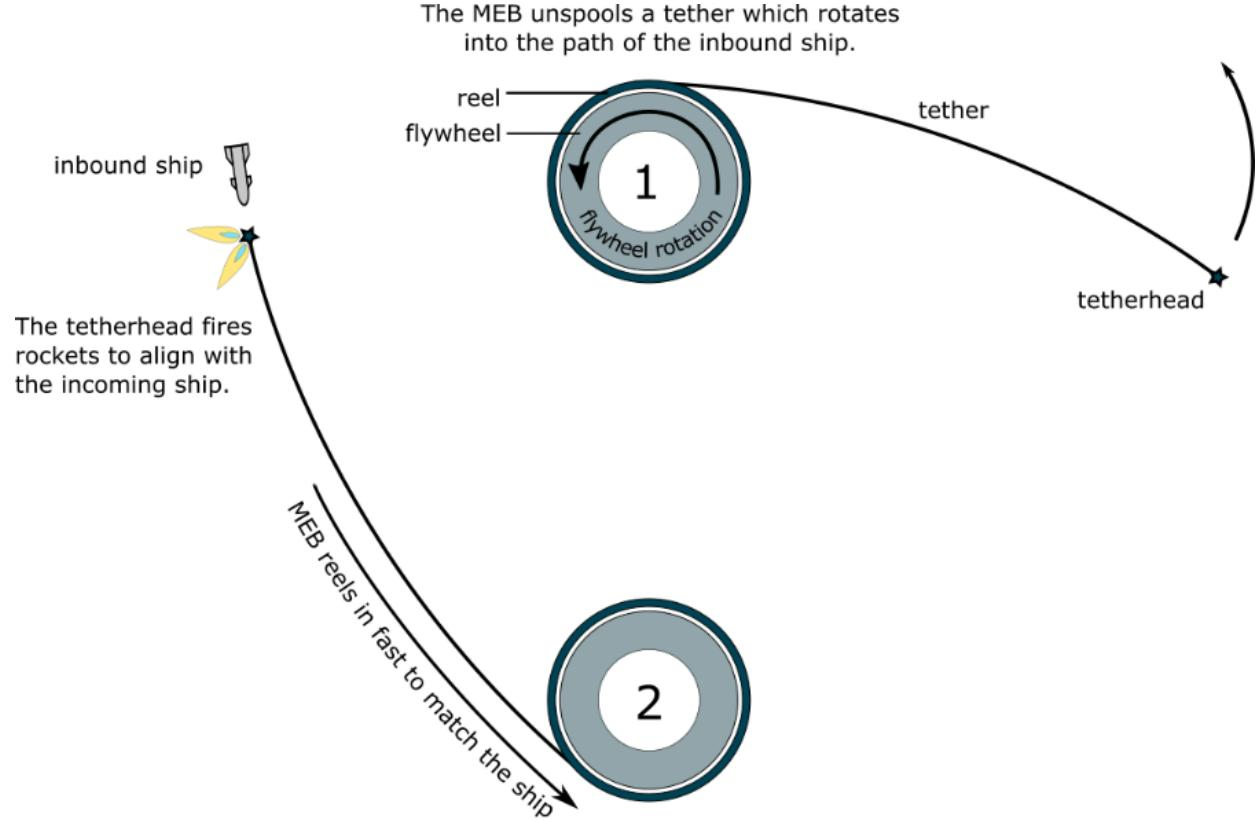
After latching the inbound ship the reel reverses direction, applying a braking force.
